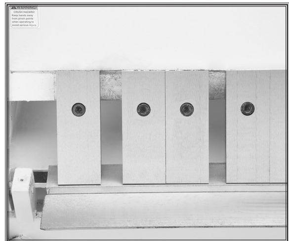
Figure 11. Fingers spaced apart to allow clearance of pan or box sides.
